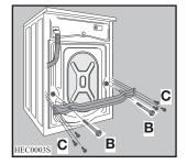
5. Remove the bracket **D** and refit the six smaller bolts C and slide out the relevant plastic spacer E.
